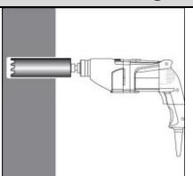
Drill with a diamond drill a hole into the base material to size and embedment depth required by the selected anchor (see table B3)
