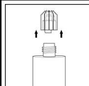
Remove the threaded cap from the cartridge.
