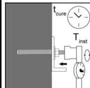
Allow the adhesive to cure to the specified time prior to applying any load or torque. Do not move or load the anchor until it is fully cured (attend Table B4). After full curing, the add-on part can be installed with up to the max. torque (Table B1) by using a calibrated torque wrench. It can be optionally filled the annular gap between anchor and fixture with mortar.
