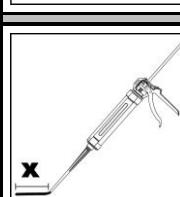
Prior to dispensing into the anchor hole, squeeze out separately a minimum of three full strokes and discard non-uniformly mixed adhesive components until the mortar shows a consistent colour. For foil tube cartridges it must be discarded a minimum of six full strokes. If you interrupt the job and restart using the same mixer inside the working time frame, discard the waste until the mortar shows a consistent colour.
