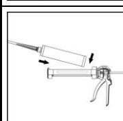
Insert the cartridge into the dispenser. Press the release trigger to retract the plunger and insert the cartridge neatly into the cradle without any distortion. Prior to inserting the anchor rod into the filled bore hole, the position of the embedment depth shall be marked on the anchor rods.
