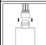
Attach the supplied mixing nozzle to the cartridge and load the cartridge into the correct dispensing tool. Cut off the foil tube clip before use if necessary.
