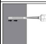
Starting from the bottom or back of the cleaned anchor hole, fill the hole up to approximately two-thirds with adhesive. Slowly withdraw the mixing nozzle as the hole fills to avoid creating air pockets. If needed, an extension nozzle shall be used. Observe the gel-/ working times given in Table B4.
