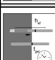
Push the threaded rod or reinforcing bar into the anchor hole while turning slightly to ensure positive distribution of the adhesive until the embedment depth is reached.
