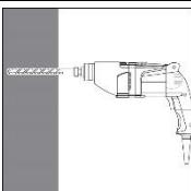
Drill hole to the required embedment depth with a hammer drill set in rotation-hammer mode using an appropriately sized carbide drill bit.(see table B3)
